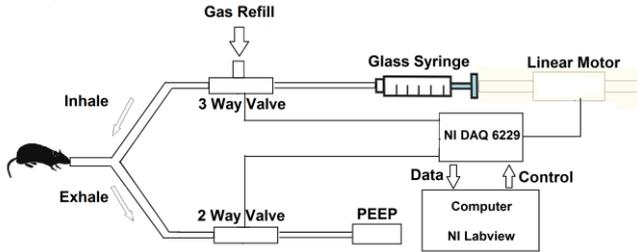
Fig. 1 Constructed mechanical ventilator's block diagram
