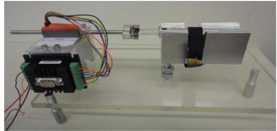
Fig. 2 Partial assembly of the mechanical ventilator, showing the connection between the linear motor's piston and syringe's plunger. Solenoid valves and tubing are not shown
