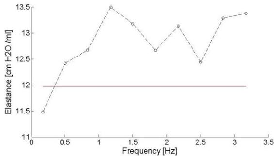
Fig. 5 Imaginary part of load's impedance divided by  $-\omega$  (elastance). Solid red line: theoretical prediction; plotted dots: experimental results.
