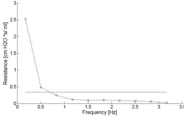
Fig. 4 Real part of load's impedance (resistance). Solid red line: theoretical prediction; plotted dots: experimental results.
