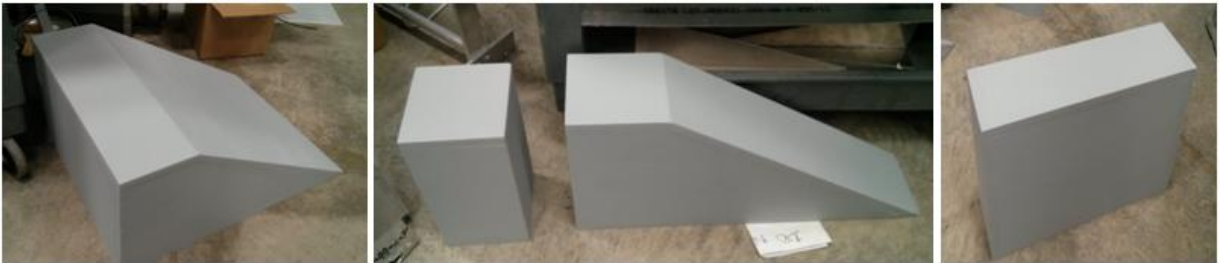
Figure 2. Physical models used for the wind tunnel experiments. All models have a height of 0.3m, and width of 0.1m (simulation of 3D flow around building) or 0.5m (simulation of 2D flow). One model has a sloped façade of 30^\circ .
